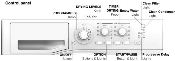
The **ON/OFF** button 0: If the dryer is running and this button is pressed and held for more that 3 seconds the dryer is turned off, the programme is then cancelled. Press and hold for more than 3 seconds and the dryer reactivates.
